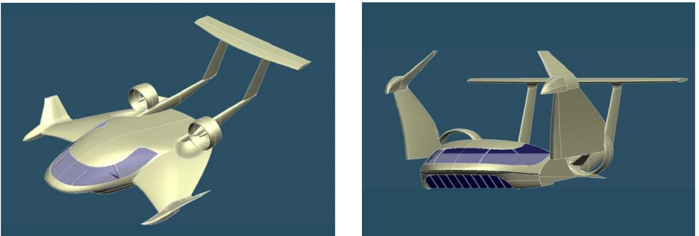
Figure 4. HW-20 showing blended/lifting body and wings folded
